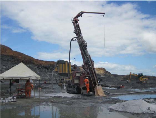
FIG 9 - Drilling operations using the PGX1350R sampling system.
