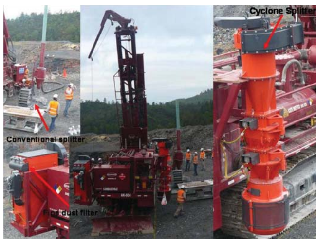
FIG 2 - (Top left) conventional Schramm cyclone with three-tiered splitter; (bottom left) S200 emission filter; (centre) drill rig with Rotaport sampling system.
